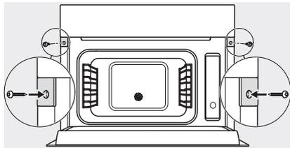
Screw joint DG DGM, installation drawing
